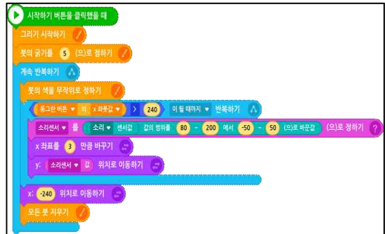
Figure 5. Code to draw a sound waveform using a sound sensor.(Blockcode the sound that the students input to the sound sensor so that it can be output as a waveform from the entry program.)
